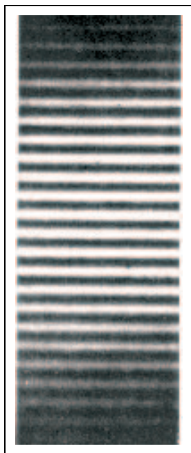
Fig. D-3: Photograph of interference maxima and minima produced by light passing through two slits.
