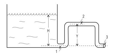
A very large reservoir is filled to a height H above a discharge outlet which sends water through a vertical loop before discharging it at point (3) into the atmosphere. Water weighs 62.4 lbf per cubic foot. At point (1), the pipe has a cross-sectional area  $A_1 = 1.00 ft^2$ , at point (2)  $A_2 = 1.00 ft^2$ , while at (3),  $A_3 = 0.75 ft^2$ .  $H = 1.00 \times 10^3$  ft and  $Y=7.0\times 10^1\,{\rm ft.}$  The outside pressure is 1.000 atmosphere (which is equal to 2116 lbf  ${\rm ft}^{-2}).$
